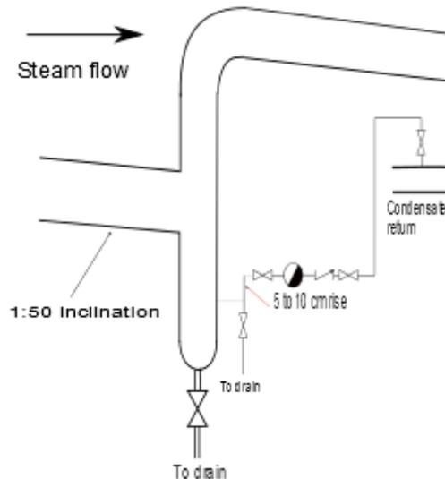
Figure 2 – arrangement for long runs
