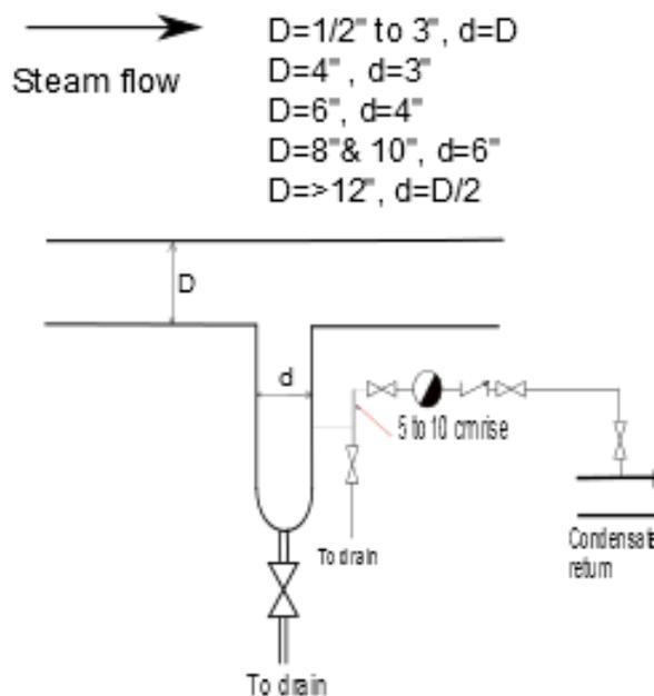
Figure 1 – typical drip leg arrangement
